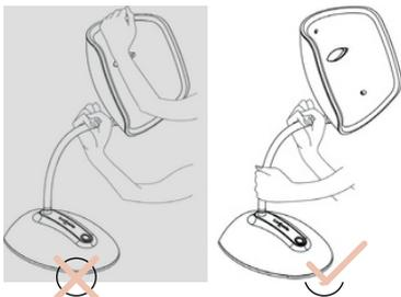
**To adjust the height of the mask, always handle the flexible cable using both hands.**
