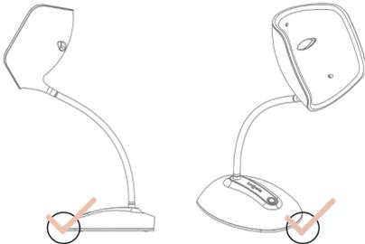
**Always turn the mask the right way around in relation to the base.** The light emitting area of the beauty mask must always be facing the front of the base. To keep the mask facing the right way with regard to the base, rotate the flexible cable.
